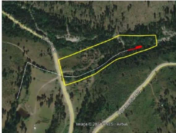
Figure 1 Basemap highlighting Shuttleworth POD infrastructure to be removed (red). The construction site (yellow) and diversion ditch (white) are included for reference
