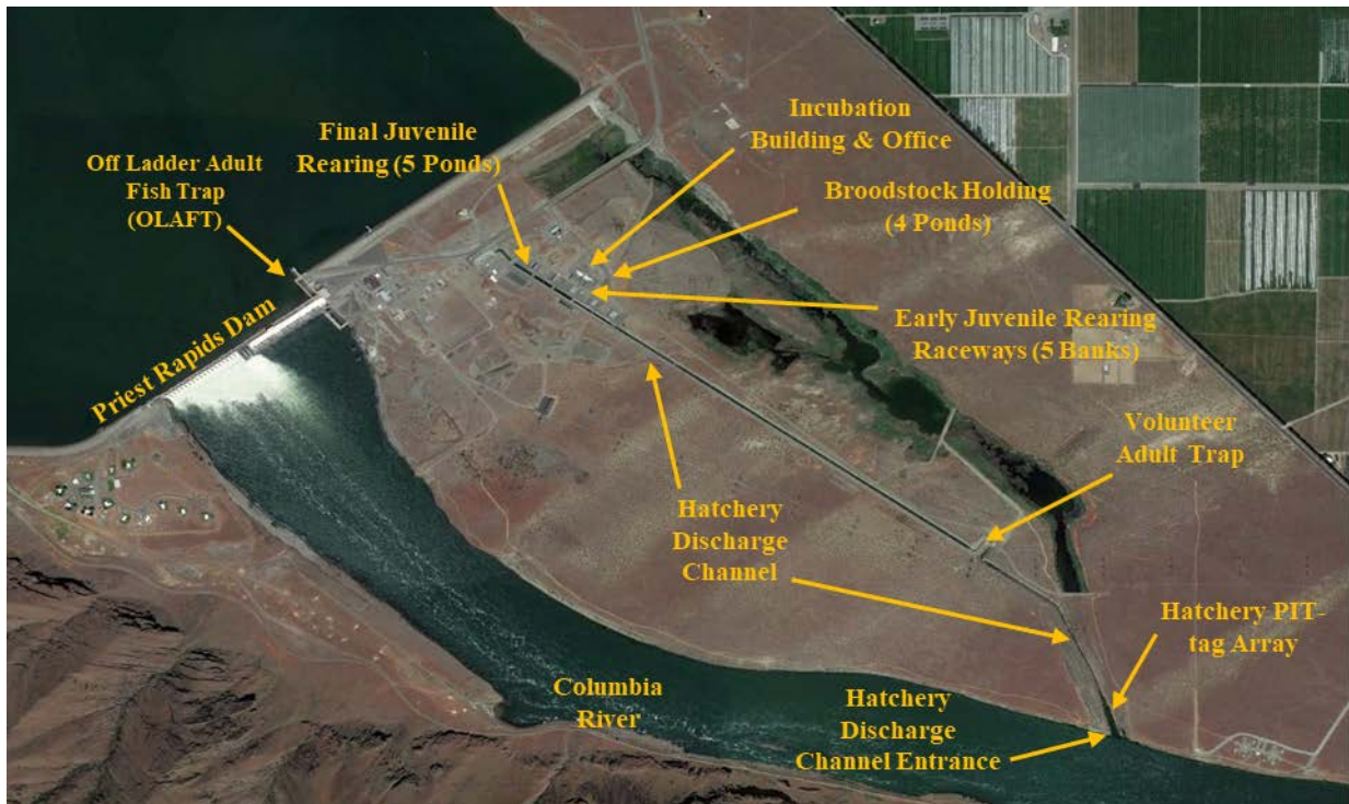
Figure 2 Priest Rapids Hatchery facility and Priest Rapids Dam Off-Ladder Adult Fish Trap (OLAFT).
