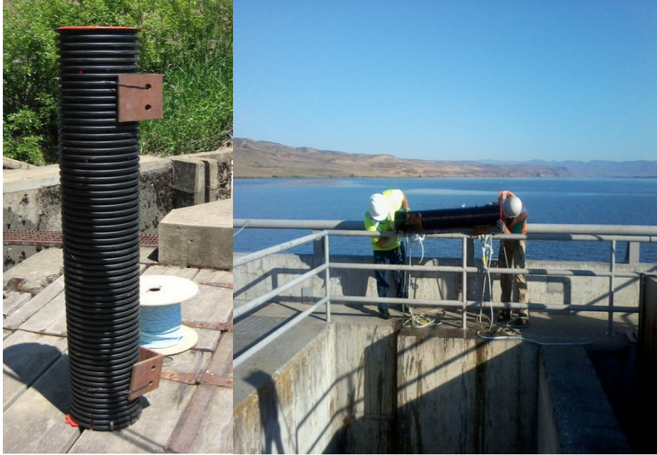
Figure 7 Adult Pacific lamprey tube traps used to collect lamprey from various locations within the fishways of Priest Rapids and Wanapum Dams, as part of the trap and transport program associated with the Wanapum Fracture.
