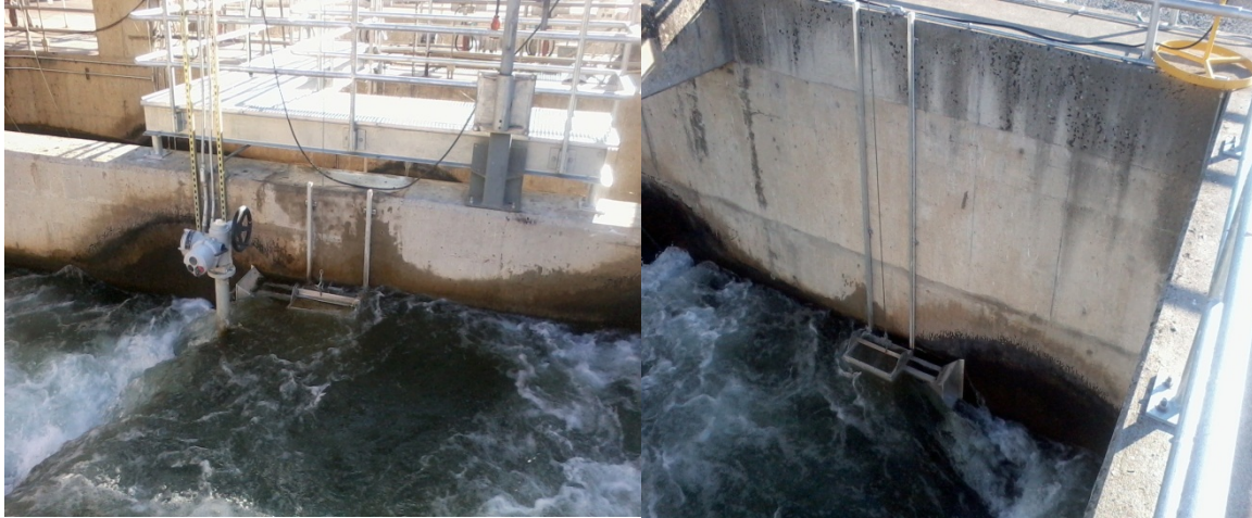
Figure 8 Fixed site adult Pacific lamprey traps located and deployed in the fishways of Priest Rapids Dam. Lamprey traps used to collect lamprey migrating through the fishways of Priest Rapids, as part of the trap and transport program associated with the Wanapum Fracture.
