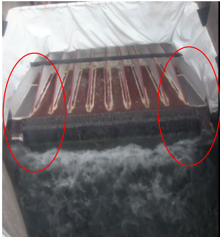
Figure 3 The Wanapum Fishway Exit Passage System (WFEPS) at the exit of the left bank fish ladder. Highlighted areas in red will be monitored with infrared-equipped high definition camcorders during the night after release of HD PIT tagged adult lamprey in the upper fish ladder in mid-July 2014.
