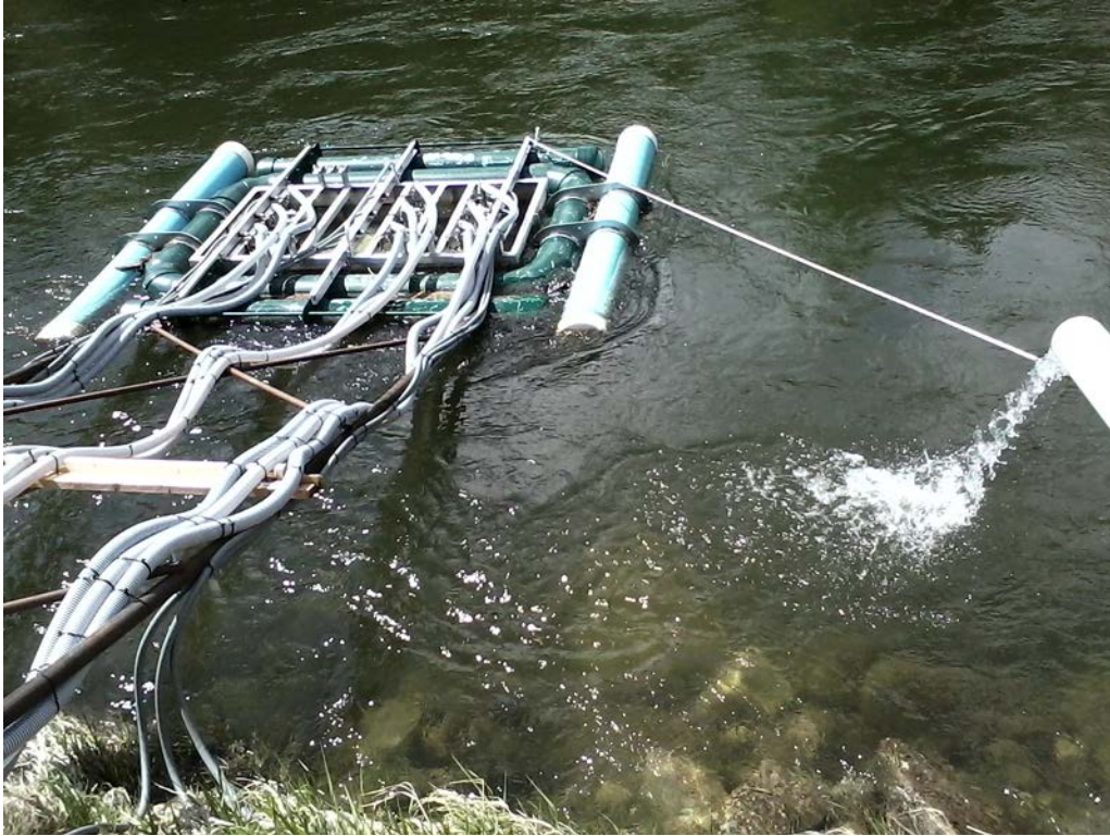
Figure 4 A photograph of the 2012 White River acclimation site water pump-basket with an outflow pipe.
