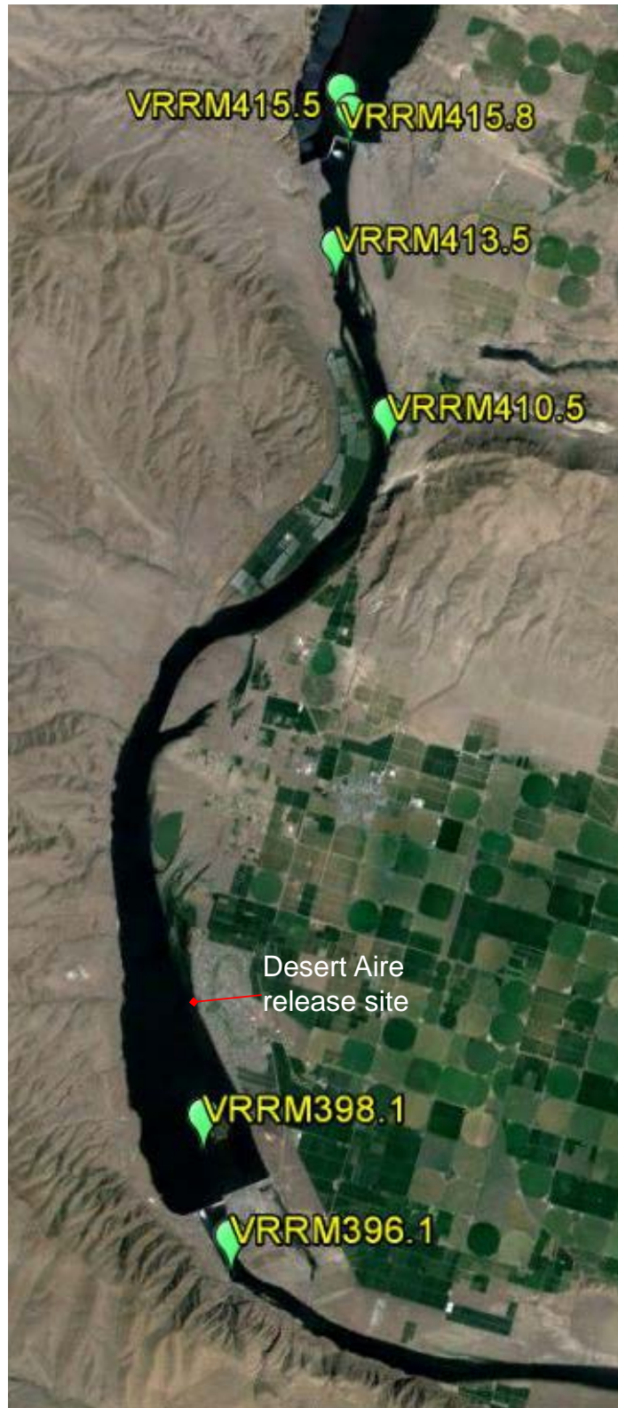
Figure 6. Locations of existing Vemco VR2 acoustic receivers in Priest Rapids Reservoir deployed for the white sturgeon monitoring program. The last four digits of each label (VRRMXXX.X) represent the river mile at the deployed location.
