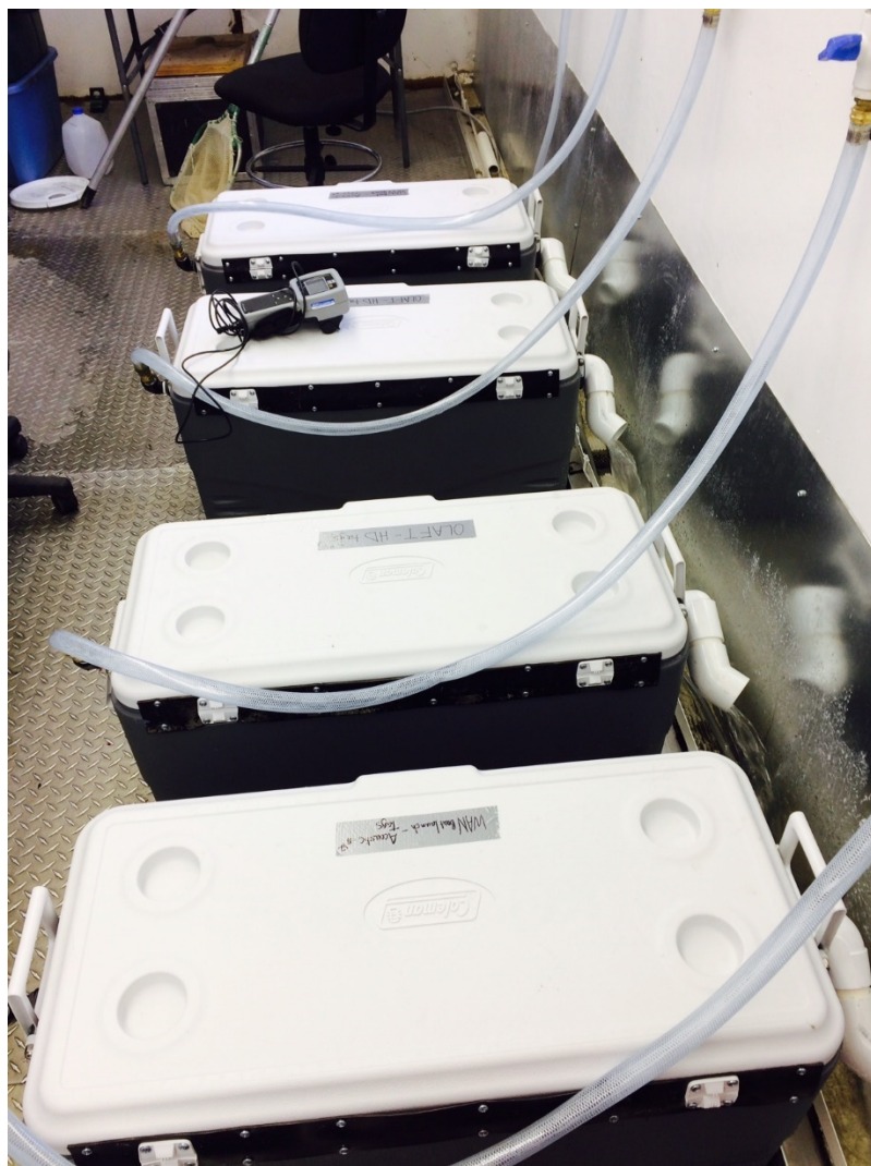
Figure 1. Holding containers (coolers) plumbed with flow-through river water at the Priest Rapids Dam left bank holding facility.
