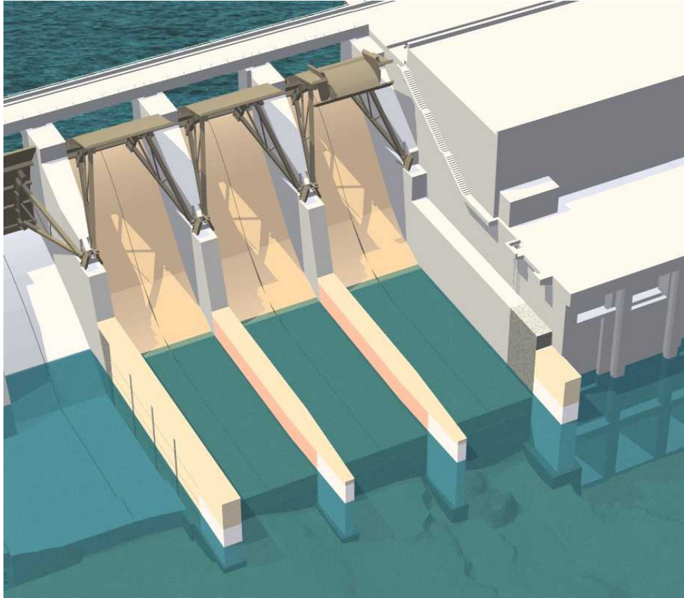
Figure 2. Graphic diagram of the Priest Rapids Fish Bypass (PRFB) showing the three bays (spill bays 20, 21 and 22, from left to right) next to the powerhouse.
