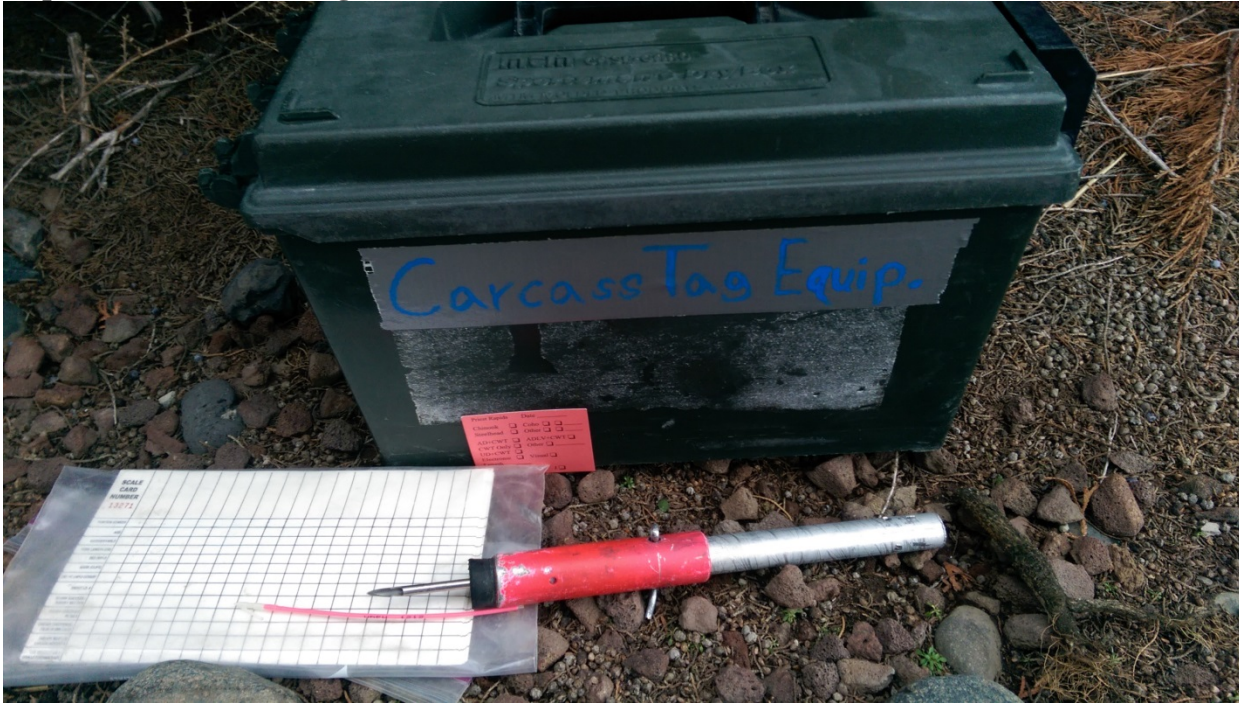
Caption 1. Picture of the pink dart tag (FT-1-94, Floy Mfg) and the aluminum application tool (Pink tube) attached to a short aluminum pole (metallic tub). The application tool was attached to a 12.5 meter aluminum pole while tagging from the boat. When possible, one tag was injected into the fish between the lateral line and dorsal fin. A second tag was injected in the opercular region of the head.
