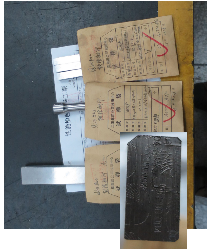
Priest Rapids hub casting material testing coupons
