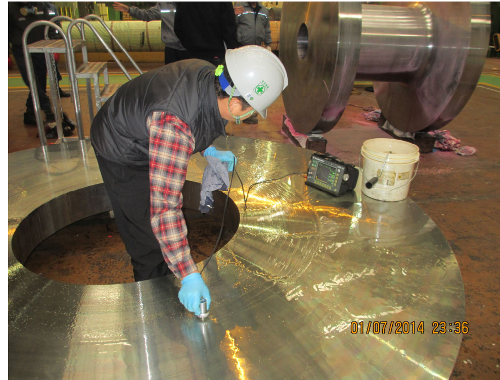
Wanapum Thrust runner forging UT inspection
