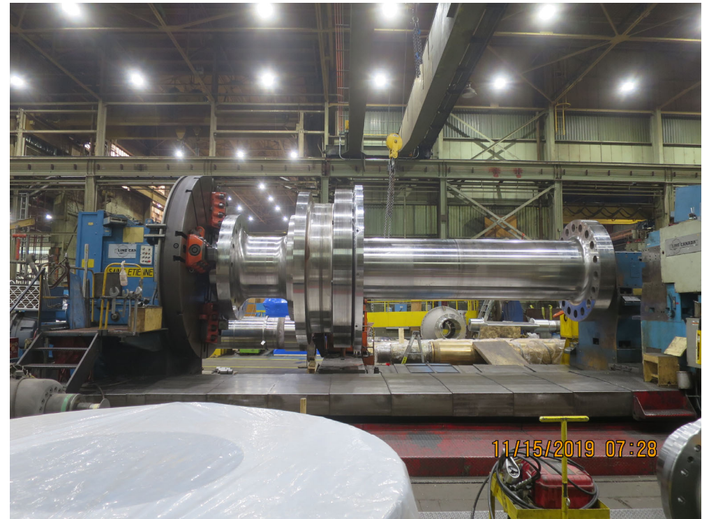
Priest Rapids generator shaft refurbishment and new thrust runner
