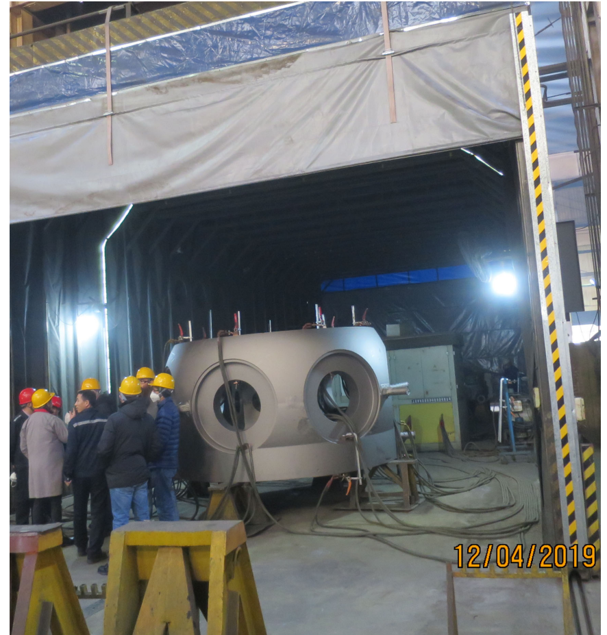
Priest Rapids runner hub casting inspection
