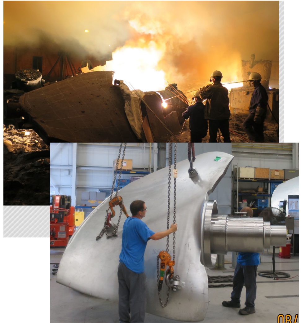
Priest Rapids turbine blade casting
